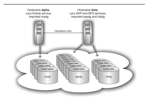
Figure 4-1: Disk groups are designed with high-availability clusters in mind. A disk group contains all storage resources for a certain service group and is dynamically imported and deported by the cluster software. During import the hostname of the importing host is written into the private region database of the disks in the disk group to prevent concurrent imports by other hosts.
